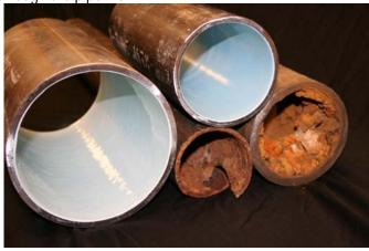
Tuberculation in the pipes can cause a substantial increase in friction loss, and can also significantly reduce the effective diameter of a pipe. This loss in diameter decreases the carrying capacity of the pipe as well as reduces the available pressure in the pipeline.
