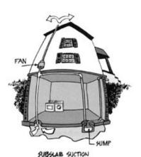
radon is usually reduced by one of four types of soil suction: subslab suction, drain tile suction, sump hole suction or block wall suction. Active subslab suction (also called subslab depressurization) is the most common and usually the most reliable radon reduction method. One or more suction pipes are inserted through the floor slab into the crushed rock or soil underneath. They also may be inserted below the concrete slab
